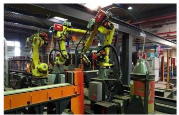
This robotic steel beam welding system is designed to fabricate most steel assemblies and accessories for structural steel buildings. Equipped with high resolution 3d scanners, the system is built to be as flexible as an assembler on the shop floor. Instead of using dedicated fixtures to make the beam straight, the BeamMaster will read the curvature and twist of the beam than simply sits on easels, and compensate both the Pick & Place and welding operations based on the normal distortions.
