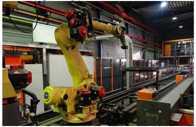
Made for W beams, HSS closed rectangular sections, Channel beams or U beams. Welding corner joints, fillet tee & lap joints, butt, v-groove, half-groove, u-groove & groove butt joints.
